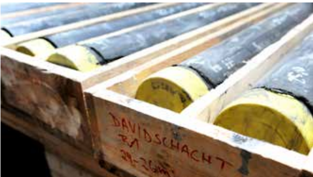
Drill cores from the Davidschacht tailing dump, Freiberg (HIF)
